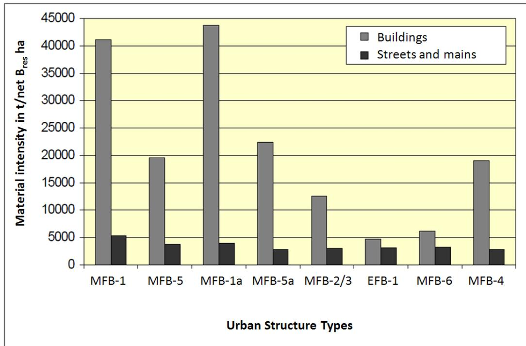
Figure 1 Material intensity of different urban structure types; comparison of buildings / streets and mains (average values for three cities in Saxony; source: IOER)
